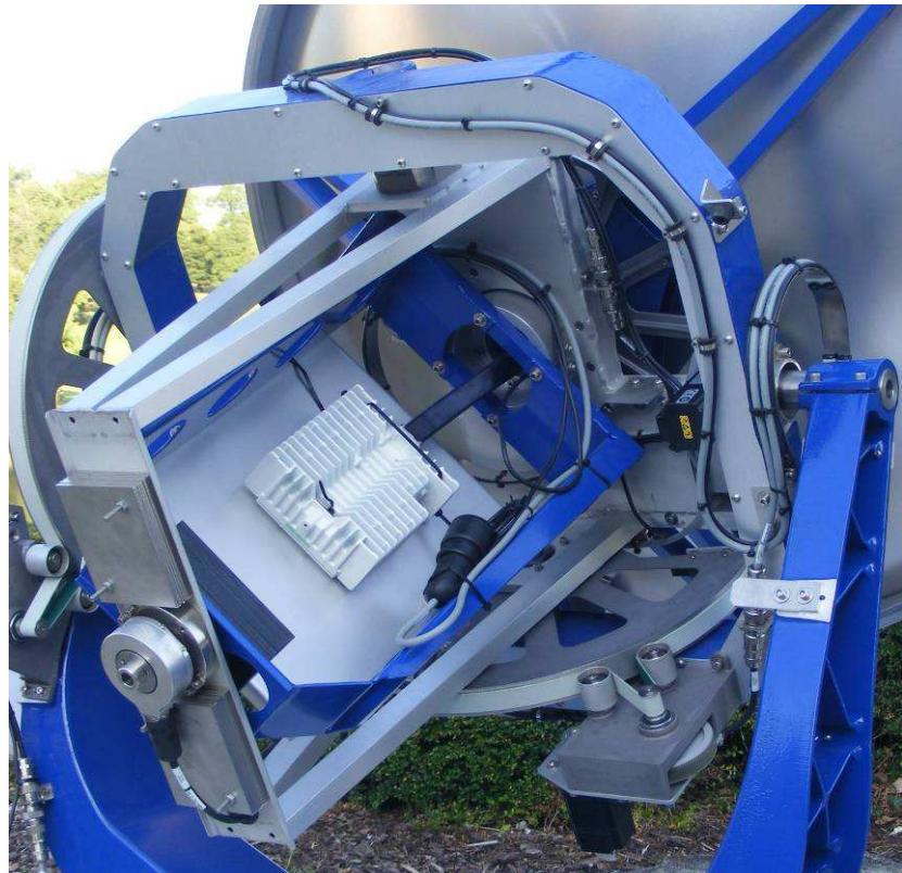
View to the chassis carrying the BUC/amplifier
