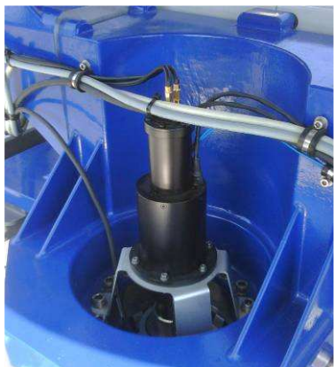
Rotary Joint for Tx/Rx cable
