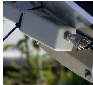
Fixing LNB with wire straps
