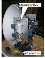
modem, most time. Nevertheless more powerful BUCs can be used and fixed, as long as they extended no maximum dimensions and weight and can be mounted (see also below the figure, where the BUC is located in the system). Be aware that for this kind of antenna system a new balancing of weight is needed every time the original balance in weight will be changed. If the
